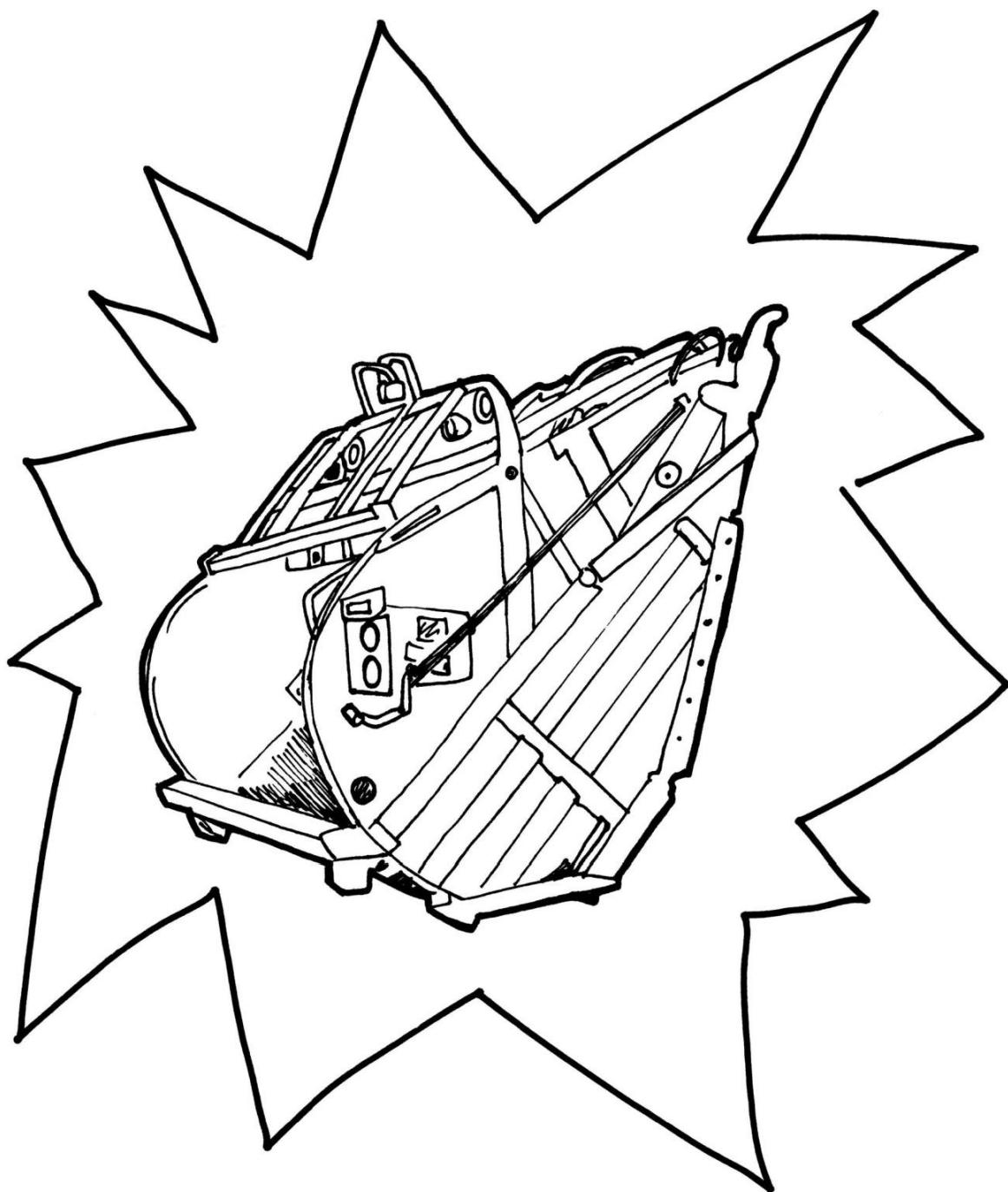
A tailgate which is the back part of the rear load truck that the trash is thrown in.
