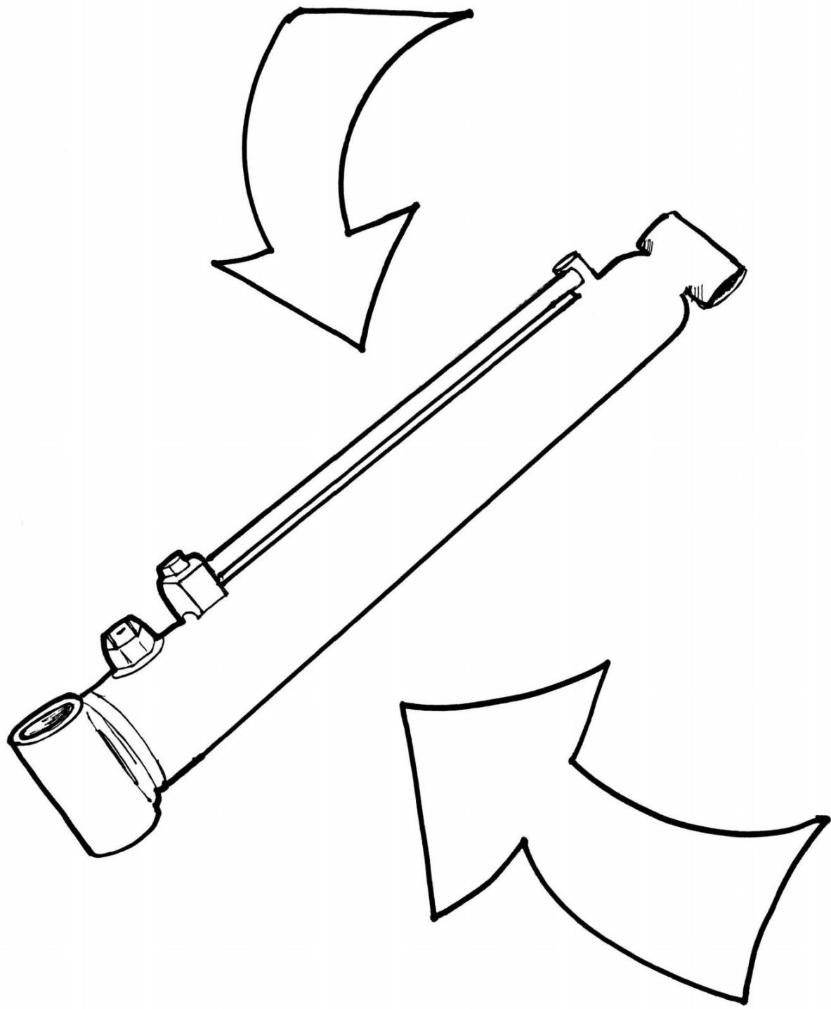
Cylinders which open the doors and lift the body.
