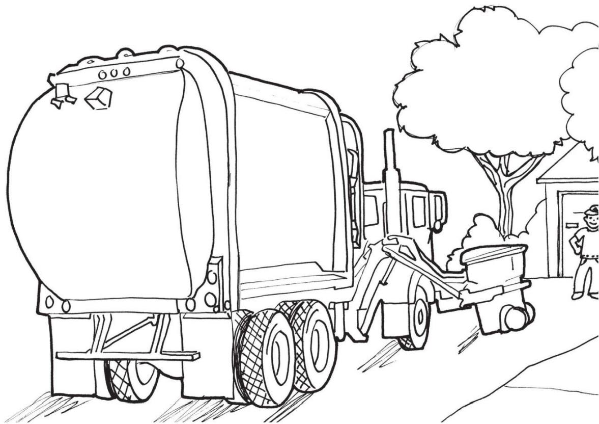
This is an automated side loader. It is loaded from the side. It has an arm that swings out and picks up the can. The driver stays in the truck.
