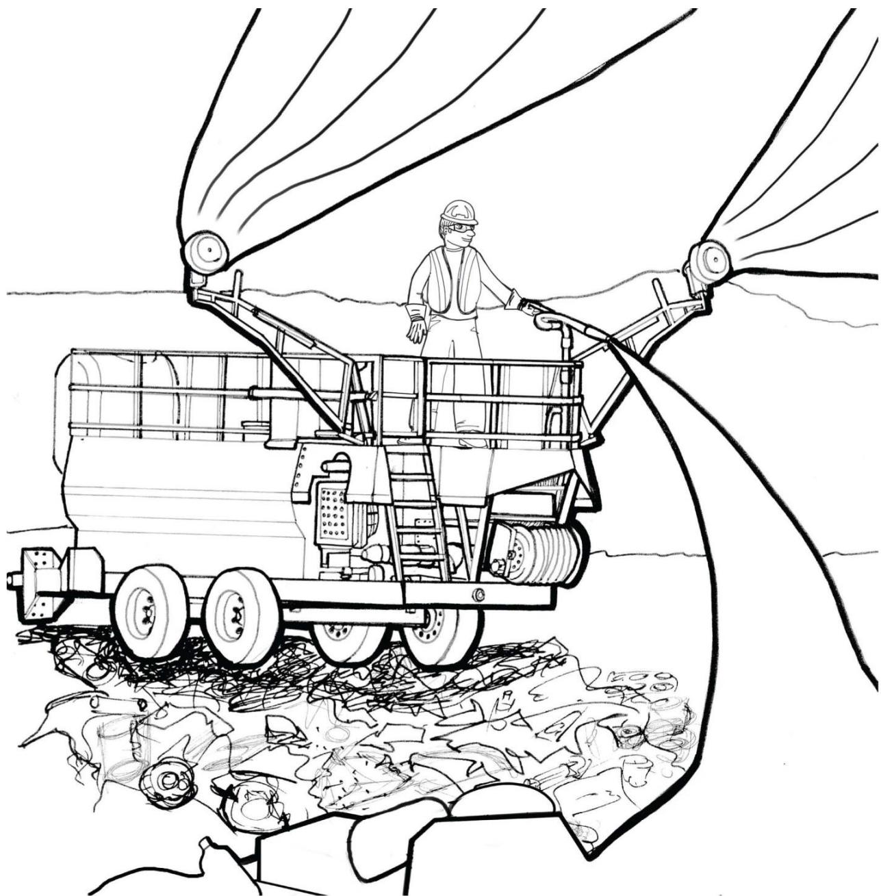
Landfills space can be saved by using recycled cellulosic materials as a daily cover. And misting naturally occurring bacteria and enzyme can reduce odors in landfills.
